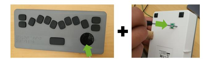
2. Connect to a PC using a USB C cable
